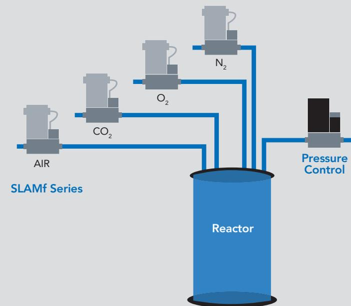
*Gas usage monitoring installation using
