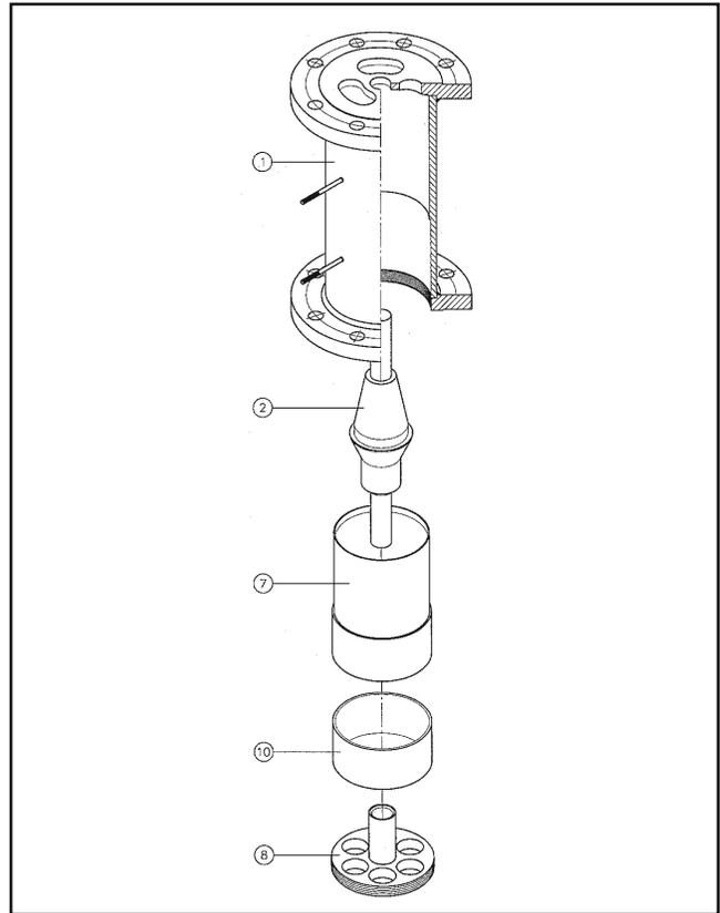
Figure 4-4 Exploded View, Model MT3809G, Size 16
