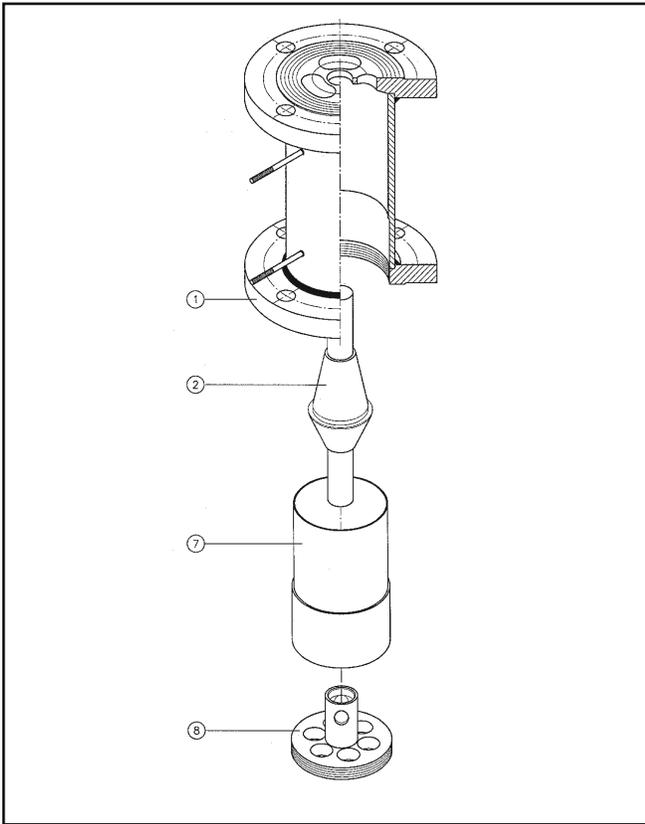
Figure 4-3 Exploded View, Model MT3809G, Size 15
