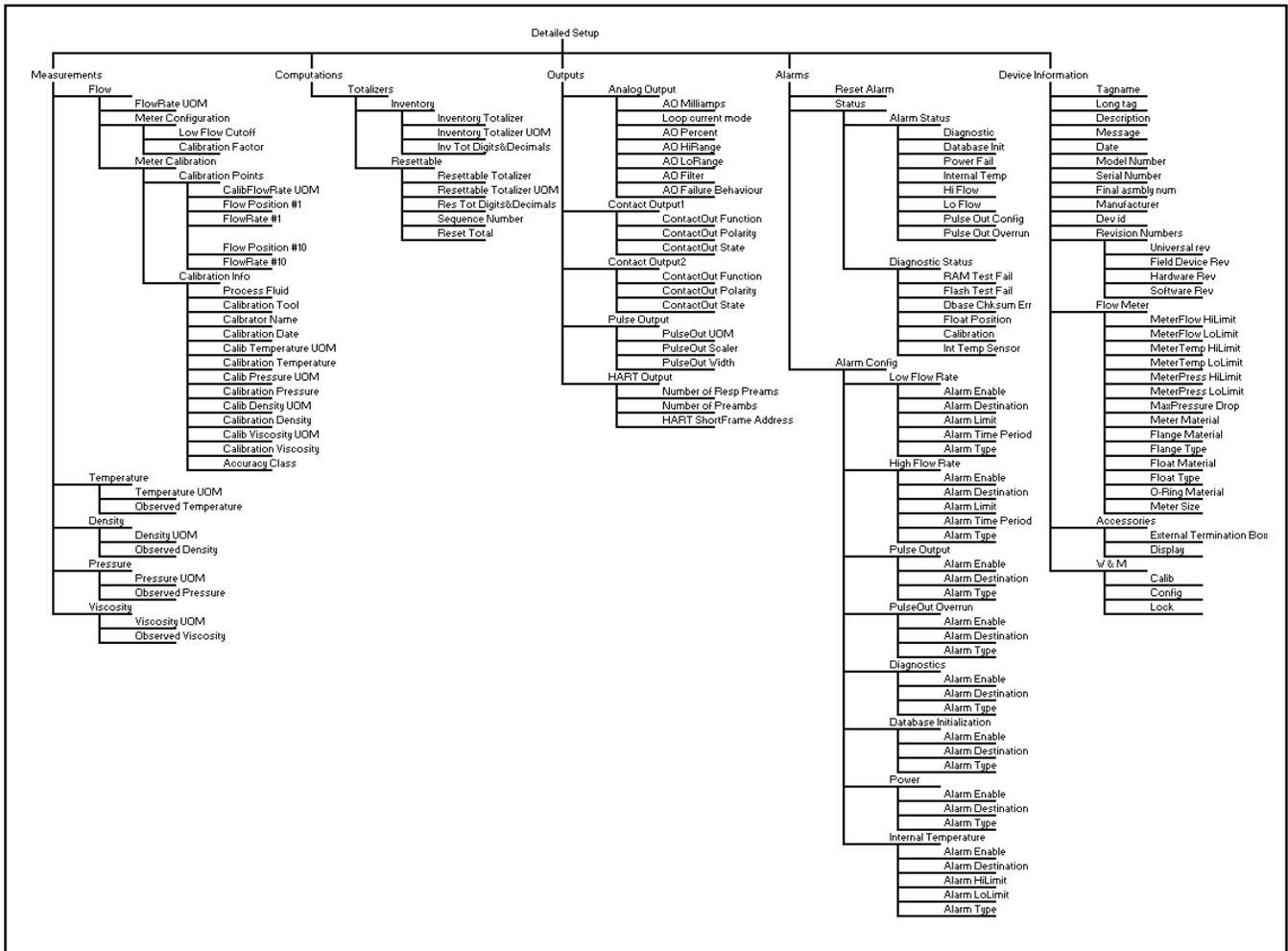
Figure 3-2 Model MT3809 Electronics Detailed Setup Menu Tree
