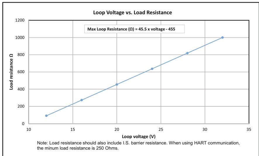
Figure 2-2 Power Supply vs. Maximum Load Resistance
