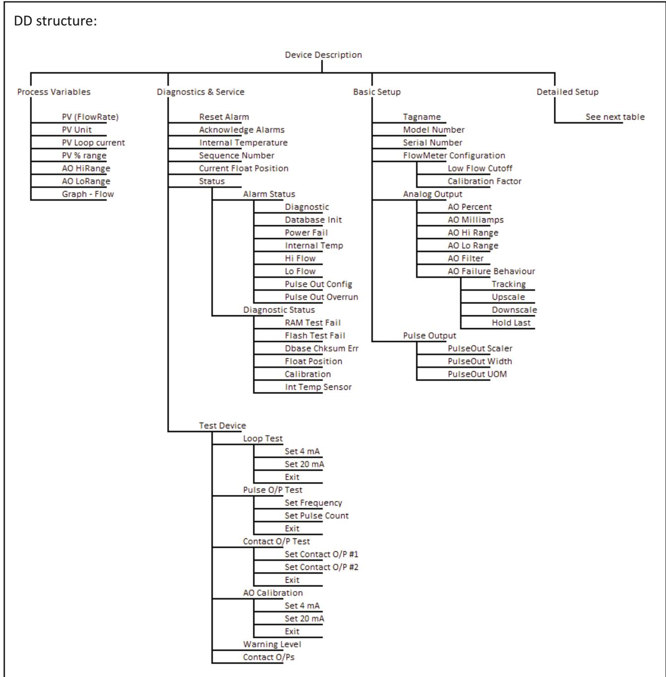
Figure 3-1 Model MT3809 Electronics Basic Setup Menu Tree
