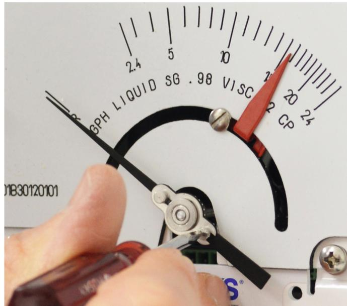
Using a flat blade screwdriver with a 1/8" blade, hold the pointer and turn the screw to align with the "R" on the scale.
