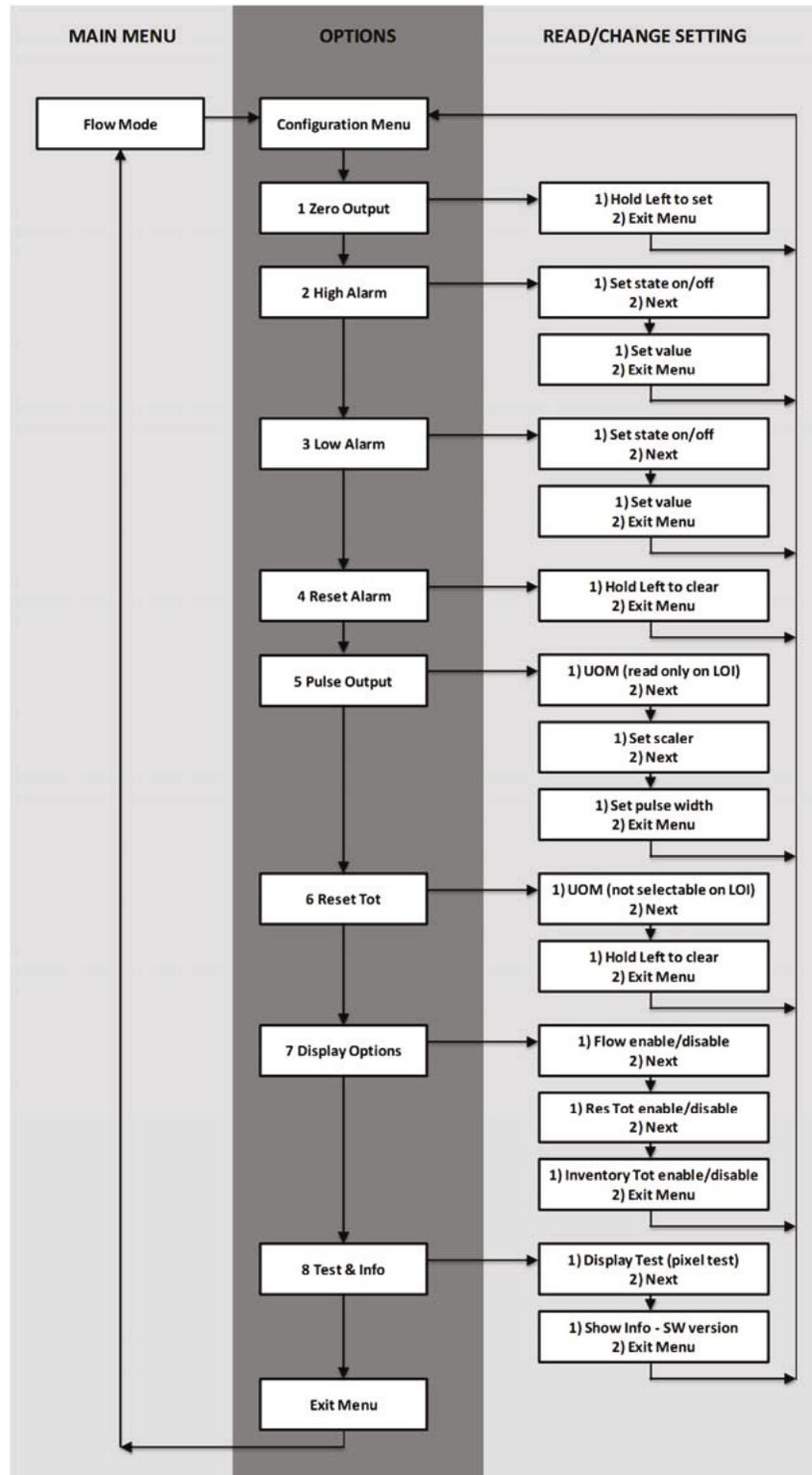
Figure 3-4 Model MT3809 Electronics LOI Chart Menu
