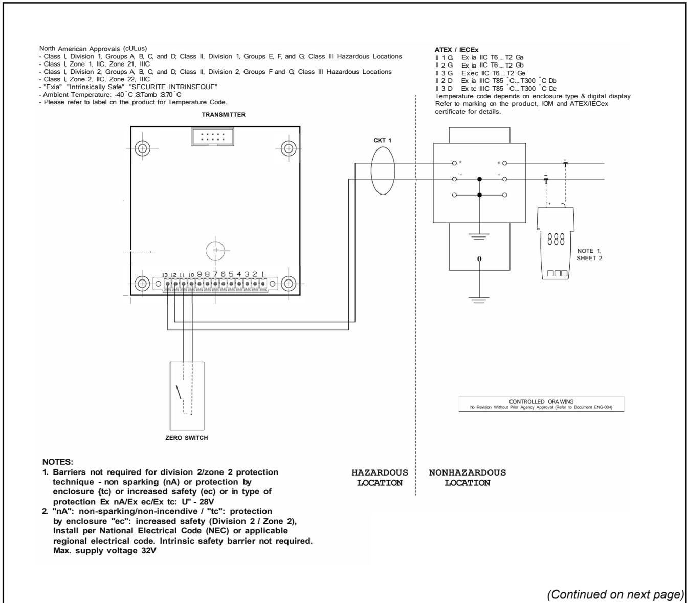
Figure 2-5 Wiring Diagram, Model MT3809 Transmitter, 4-20 mA
