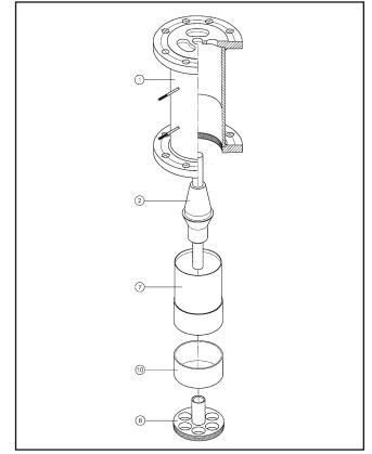
Figure 4-4 Exploded View, Model MT3809G, Size 16 (Liquid Service Only)
