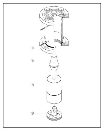
Figure 4-3 Exploded View, Model MT3809G, Size 15 (Gas or Liquid Service)
