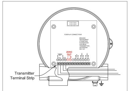
Figure 2-11 FOUNDATION Fieldbus Transmitter Indicator Zero
