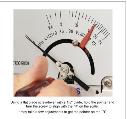
Figure 2-3 Mechanical Indicator Zero
