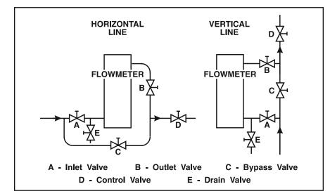
Figure 2-1 Typical Bypass Installation
