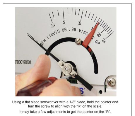
Figure 2-10 Mechanical Indicator Zero
