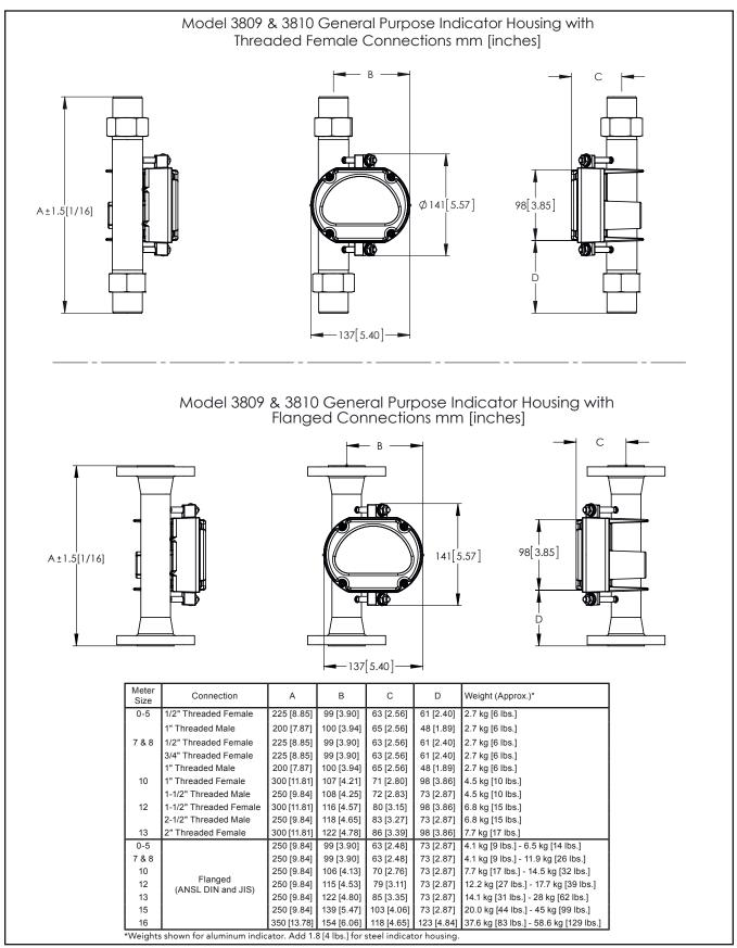
Figure 1-1 Model MT3809 and MT3810 Dimensional Drawings (mm/in) and Weights (kg/lbs) - General Purpose Housing
