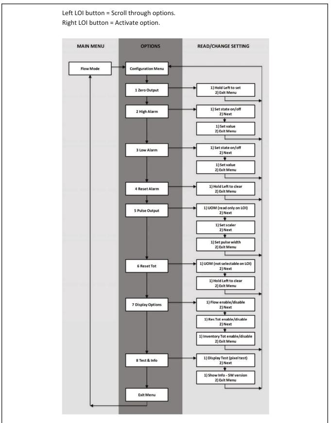
Figure 3-4 Model MT3809 Electronics LOI Chart Menu
