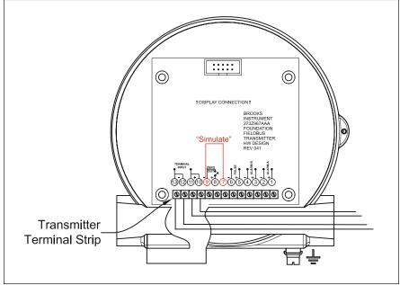
Figure 3-3 Transmitter "Simulate" Connection
