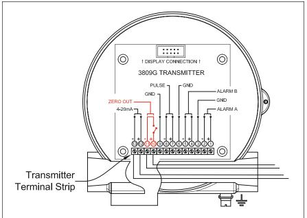
iii. Then, zero the transmitter shorting the two pins at the terminal block. Reference Figure 2-4 below.
