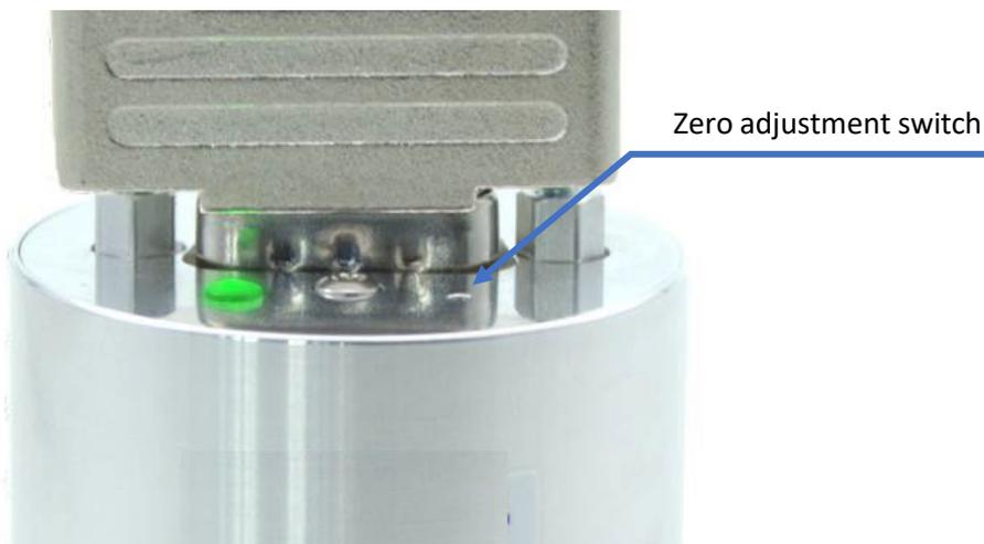
1. Evacuate the gauge to a vacuum pressure below 1.00E-6 mbar.
