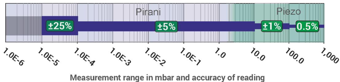
The MEMS-Pirani provides measurement resolution down to 1.00E-6 mbar (7.5E-7 Torr).
