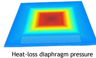
The piezo MEMS sensor consists of a diaphragm where one side of the diaphragm is exposed to the vacuum gas and the other side is exposed to a sealed reference vacuum. The applied pressure deflects the diaphragm, and the deflection is converted to an electric signal.
