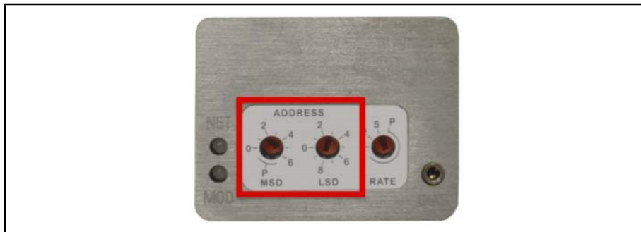
Figure 3-2 MAC ID Switches
