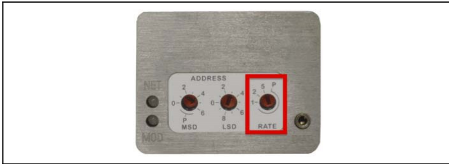
Figure 3-1 Baud Rate Switch
