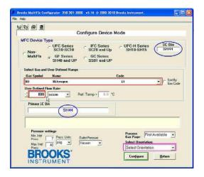
12. As the software reads the device calibration and writes a new process gas page to the device the status will show progress. When complete the Configuration Completed screen will appear. A new Customer Part Number can be entered into the unit. Top Labels can be printed for the new configuration or you can view Details of some older configurations in the device. When completed click Return to go back to the Main screen. The network will be rescanned to update the scan list.
