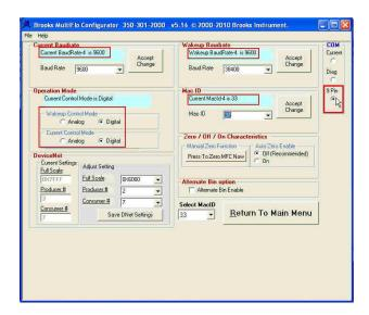
16. To configure the mass flow controller or meter for the most common RS485 digital communication settings select:
