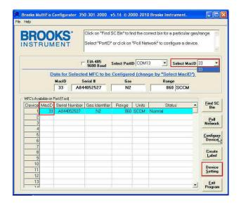
14. To view the current DeviceNet configuration note the Full Scale, Producer # and Consumer # settings of the DeviceNet – Current Settings section. To adjust the DeviceNet settings to match the tool configuration select DeviceNet – Adjust Settings – Full Scale, Producer# and Consumer# Common configurations are:
