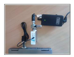
9. From the MultiFlo Configurator main page select the communication port used to connect between the device and PC (**Select PortID**). If using a USB-COM port adapter or USB-RS485 adapter, these must be connected before starting the MultiFlo Configurator software. Click **Poll Network**. The following status messages will be displayed:
