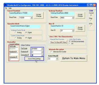
15. To view the current RS485 configuration for the 9 pin connector select **9 Pin** and note **Current BaudRate**, **Wakeup BaudRate**, **Control Mode** and **Mac ID**.
