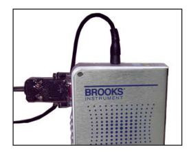
8. Connect communication cable. There are various ways to connect the device regardless of device configuration. Devices may be connected through the diagnostic port using cables in the Basic MultiFlo Configurator Kit (P/N 778Z010ZZZ) for RS485 communications.
