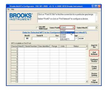
10. If there are multiple devices connected to the bus a short summary will appear in the MFCs Available on Port(Tool) section listed in MacID order. Select MacID drop down list box will automatically display the first available device but can be changed to any desired device on the connected bus. Click on Configure Device to proceed to the configuration page.
