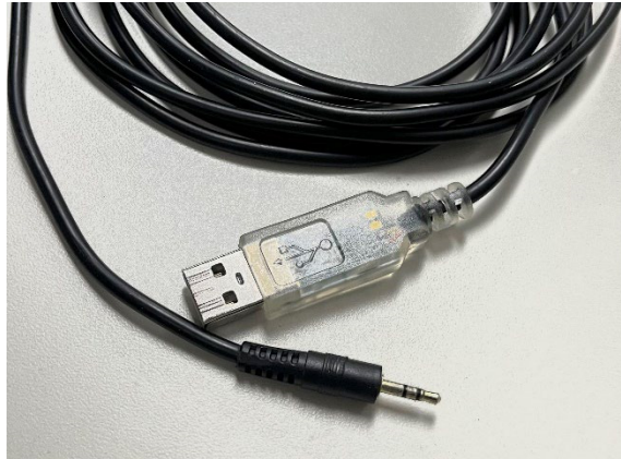
Figure 2-1 USB to RS-485 Converter, cable included in Basic Cable Kit 778Z010ZZZ (2.5-mm jack plug to USB Type A Plug)
