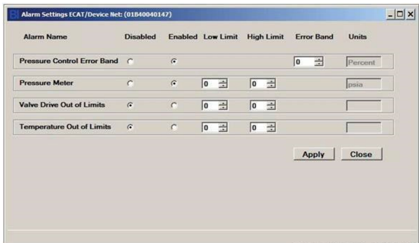
Figure 11-25 Alarm Settings DeviceNet/EtherCAT Window (Exact alarms settings available varies depending on device type)
