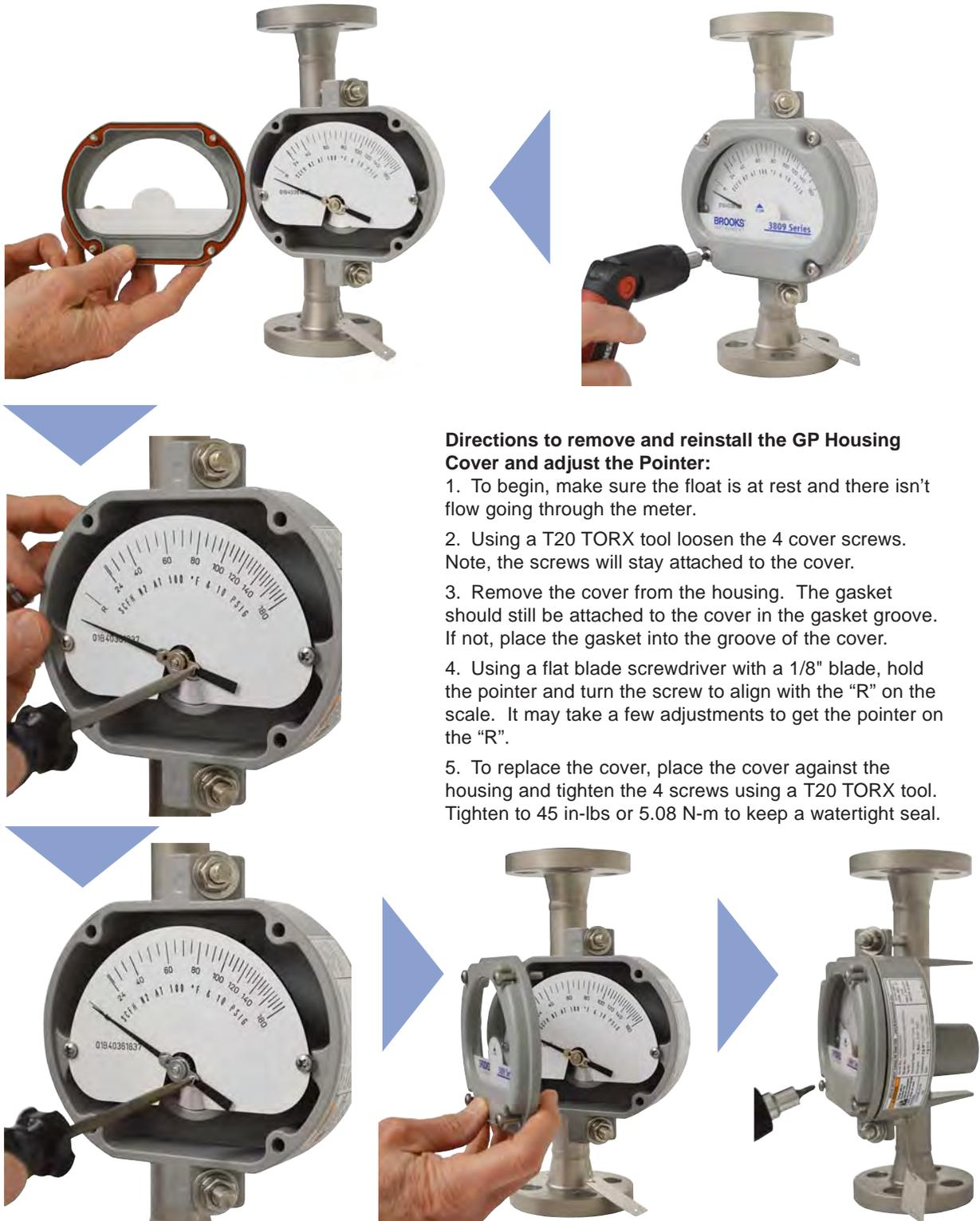
**Directions to remove and reinstall the GP Housing Cover and adjust the Pointer:**
