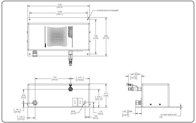
Figure 2 Dimensions - DLIHV 3000 Watt
