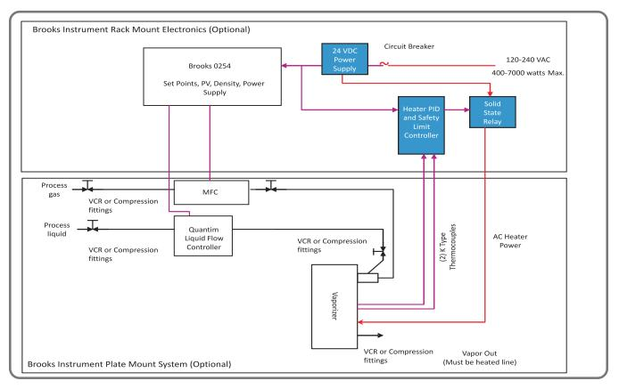
The most common integrated system is a plate-mount system consisting of the DLIHV heat exchanger mounted on a brushed stainless steel or aluminum backplate, along with the Brooks' Quantim® Coriolis liquid mass flow controller and a Brooks' carrier gas thermal mass flow controller. Optional components include a pneumatic liquid shutoff valve, the Brooks' SolidSense II pressure transducer or the Brooks' XacTorr® CMX Series digital vacuum capacitance manometer.
