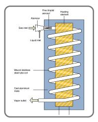
The DLIHV circulation heater is constructed of a 316L stainless steel helical coiled tube cast in an aluminum body with tubular elements. The aluminum body serves as the heat transfer media between the tubular heating elements in the center of the heater and the coiled tube through with the fluid passes. The aluminum casting around the stainless steel tubing increases the thermal mass ensuring accurate temperature control of the fluid so as to prevent thermal degradation.
