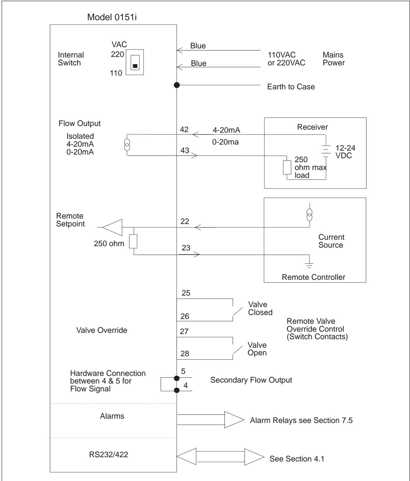
Figure 7-4 Connection Between Model 0151i and External Equipment
