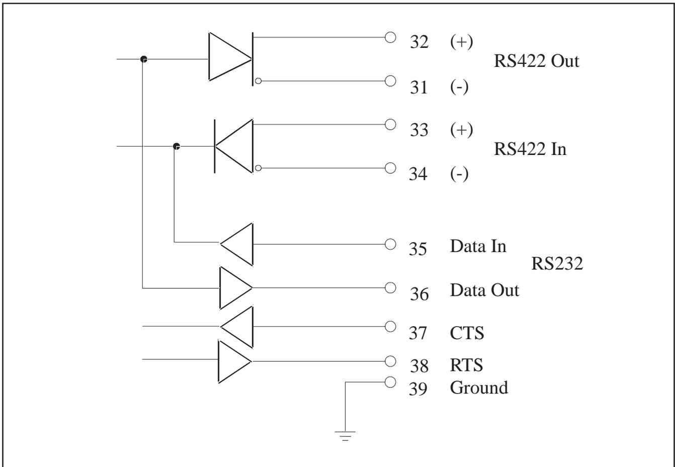
Figure 4-1 RS232/RS422 Communications Hardware
