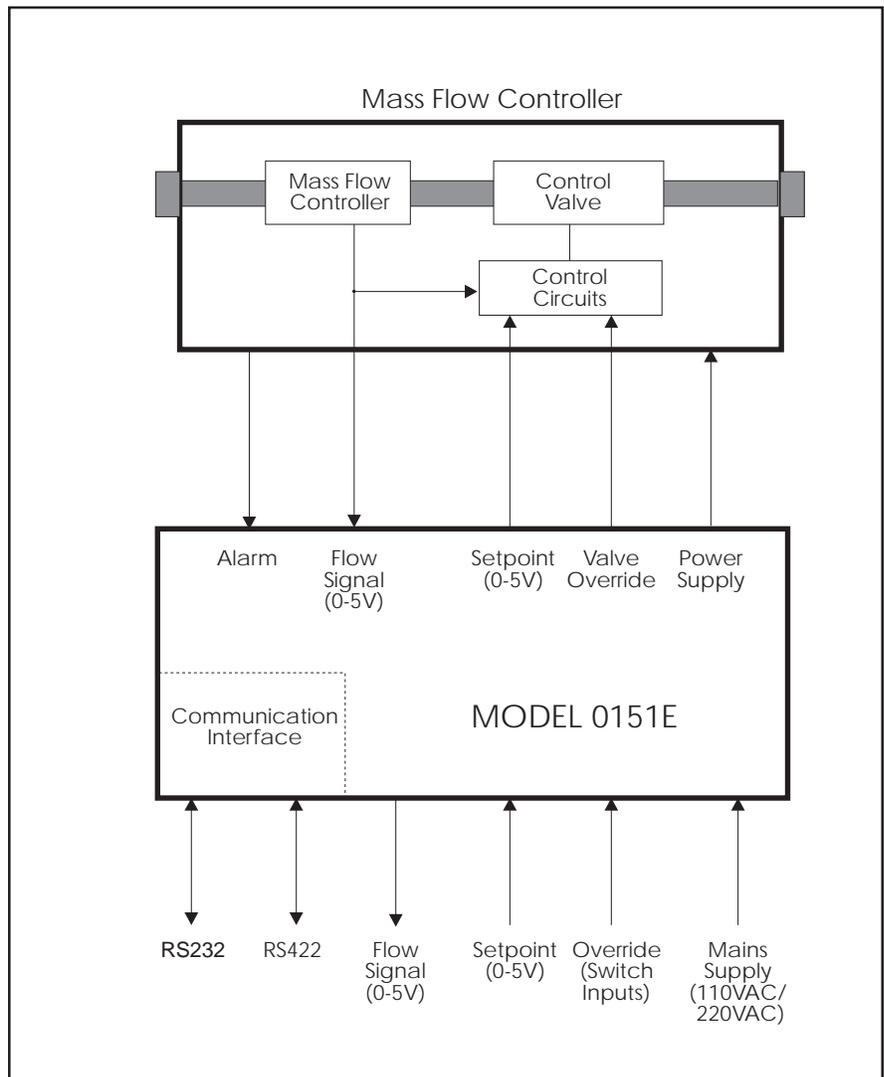
Figure 3-1 Block Diagram of the Model 0151E
