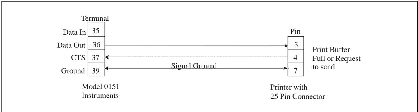
Figure 4-3 Connection to a Standard Computer Printer
