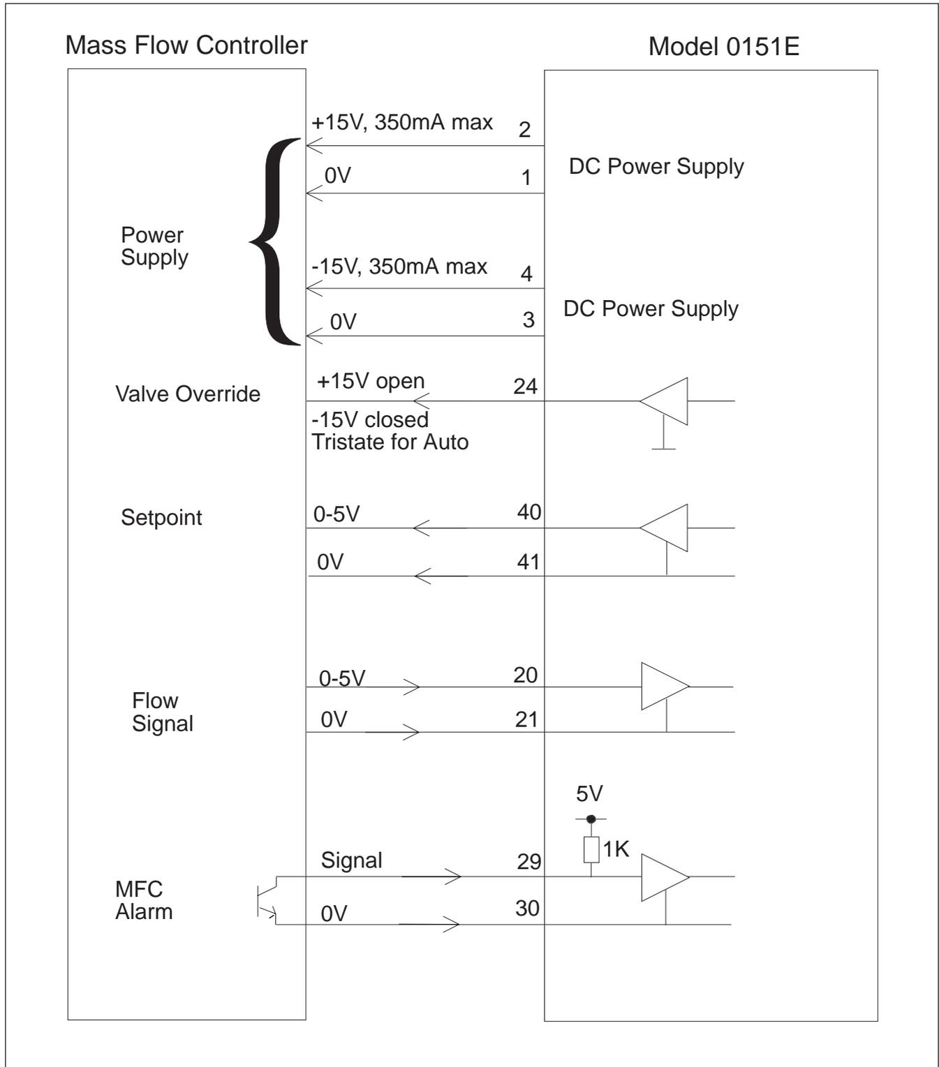
Figure 7-1 Connection Between Model 0151E and Mass Flow Controller
