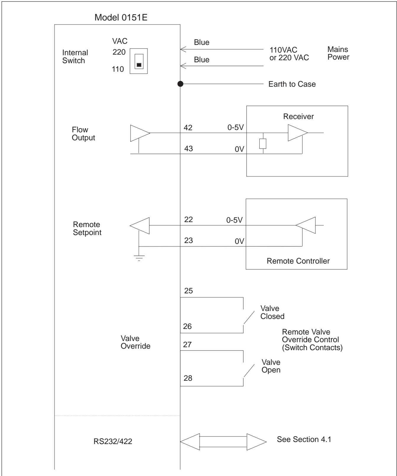
Figure 7-2 Connection Between Model 0151E and External Equipment
