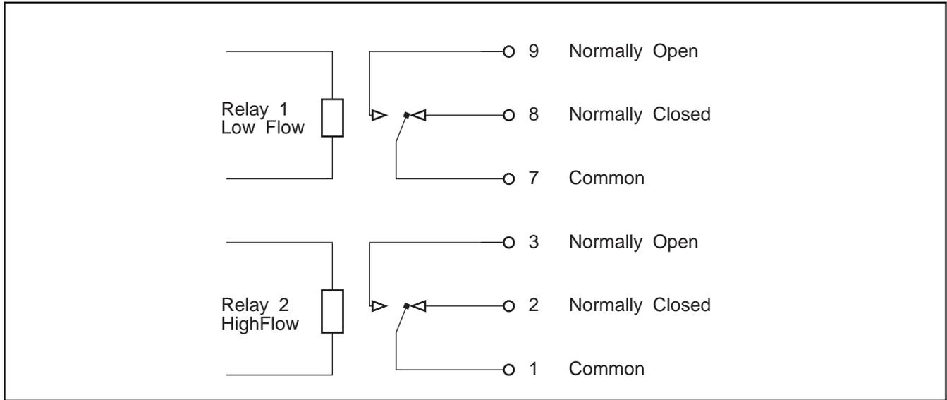
Figure 7-5 Flow Alarm for Model 0151*i* only
