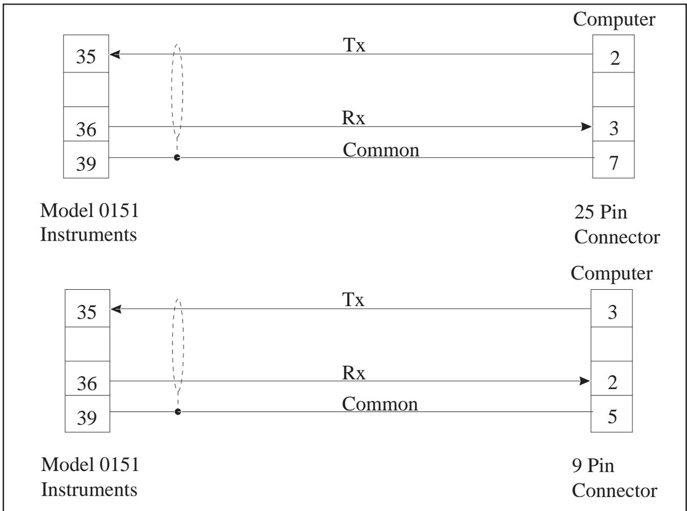
Figure 4-2 Connection to Computers with 25 Pin (Top) and 9 Pin (Bottom) Connectors
