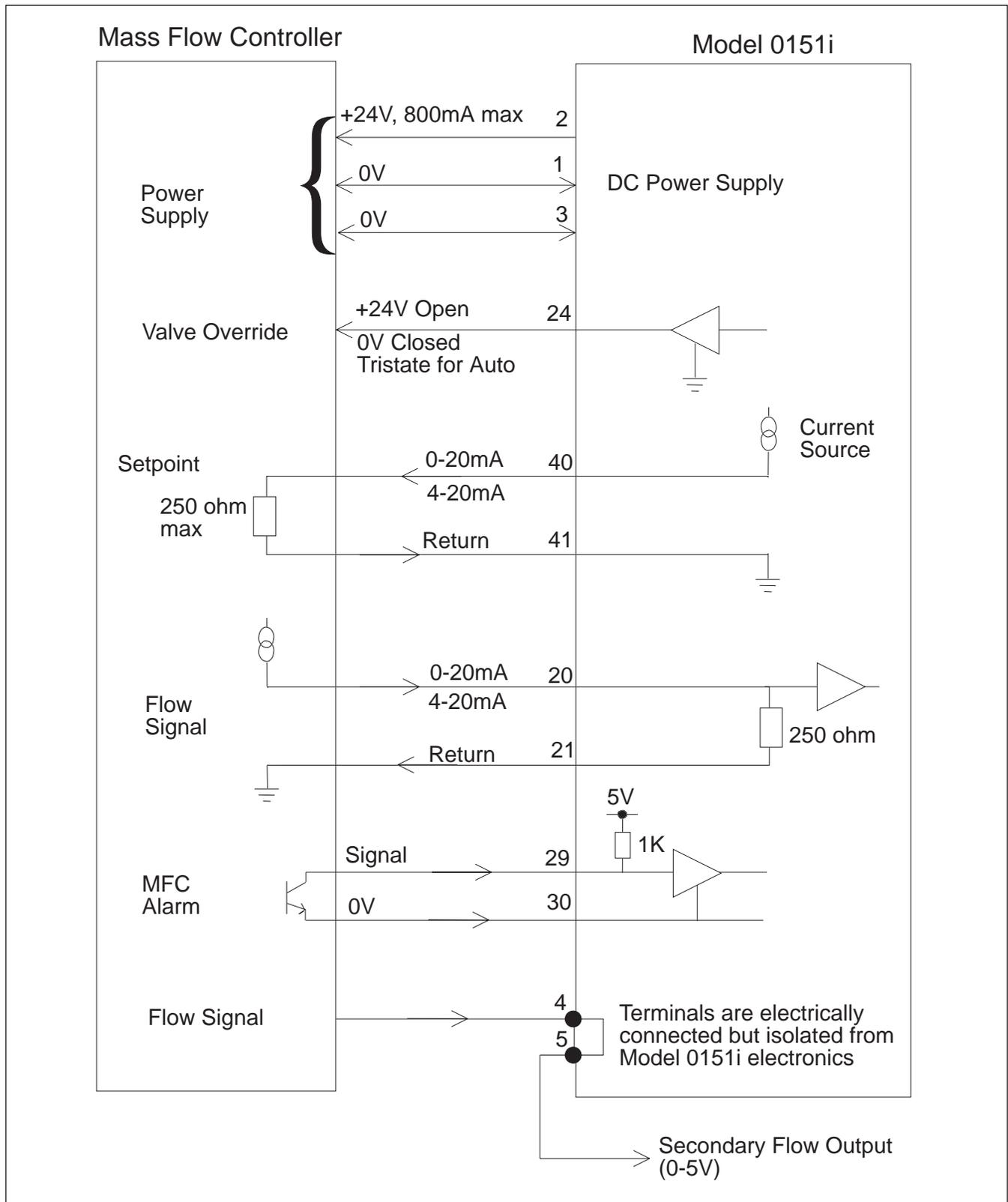
Figure 7-3 Connection Between Model 0151i and Mass Flow Controller
