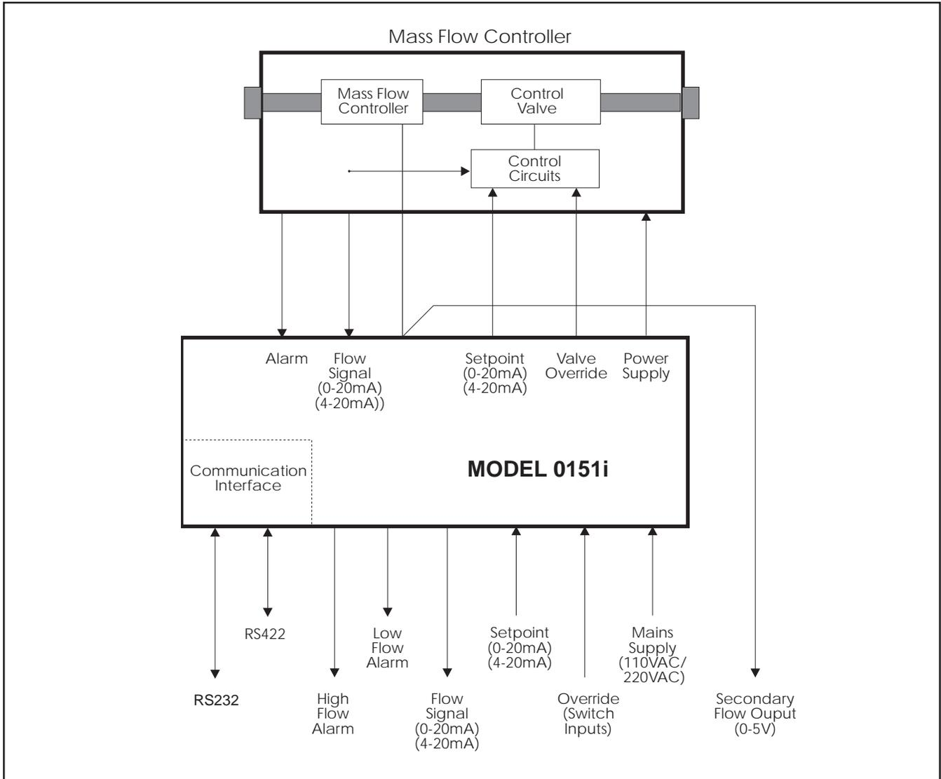
Figure 3-2 Block Diagram of the Model 0151i
