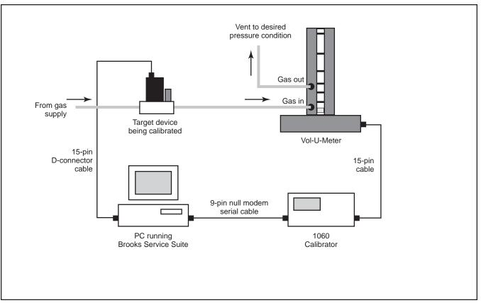
Figure 8-1 Equipment Setup for Automatic Vol-U-Meter Mode Calibration
