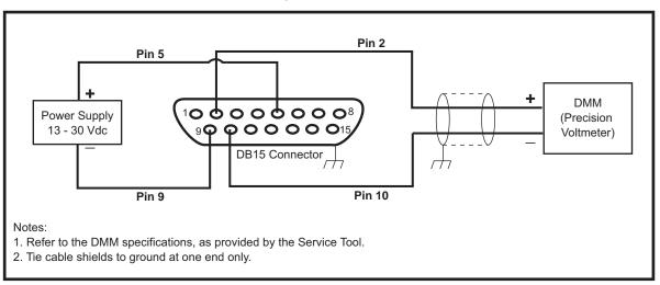
Figure 6-1 Setup for Testing Output Voltage
