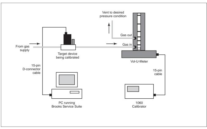
Figure 8-2 Equipment Setup for Manual Vol-U-Meter Mode Calibration
