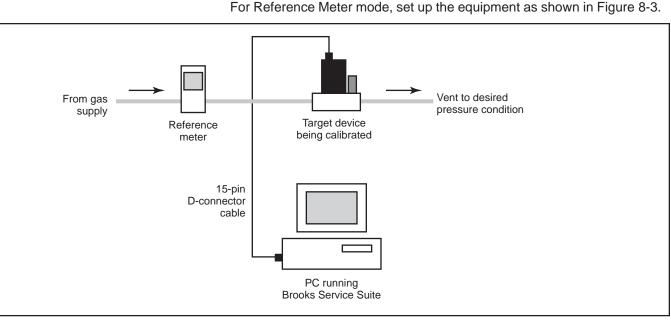
Figure 8-3 Equipment Setup for Reference Meter Mode Calibration
