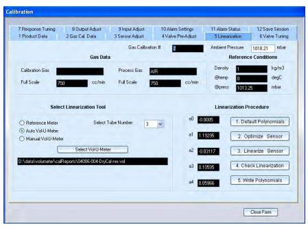
In the next series of steps, you are going to check the flow for different Data Points, but using the updated linearization polynomial. The Check Linearization process will check the results against the expected flow rates, and display deviation error values for each Data Point flow run.
