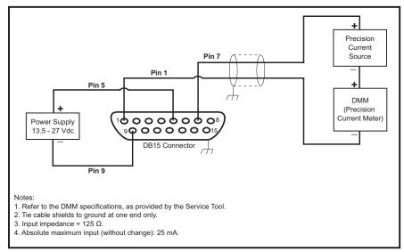
Figure 6-4 Setup for Testing Current Setpoint
