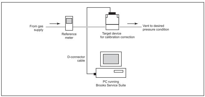
Figure 9-1 Equipment Setup for Reference Meter Mode Calibration
