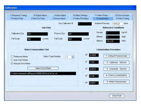
You access the calibration functions from the Linearization tab.
