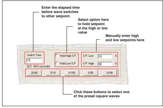
Figure 7-1 Setting Up the Setpoint Square Wave
