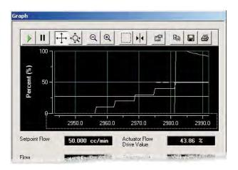
In the second adjustment phase, the setpoint is repeatedly cycled (according to the setpoint cycling values that you specified) until offset and span differences are below an acceptable threshold, or for a maximum of six cycling periods. This adjustment process can take several minutes.
