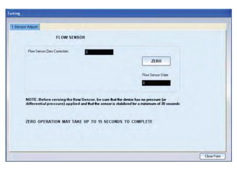
On the Sensor Adjust tab, click the Zero button. A message box displays when the zeroing operation is complete.
