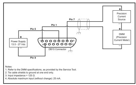
Figure 7-7 Setup for Calibrating to a Current Setpoint
