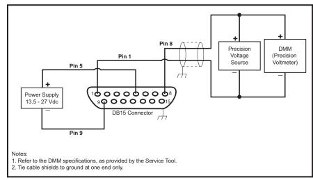
Figure 6-3 Setup for Testing Voltage Setpoint
