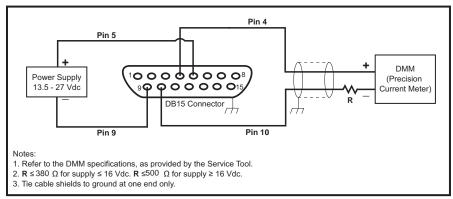
Figure 7-5 Setup for Calibrating to an Output Current
