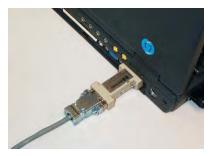
If the distance is short enough, you can connect the communications interface adapter directly to the PC's serial port, as shown below, and do not need the RS-232 serial cable.
