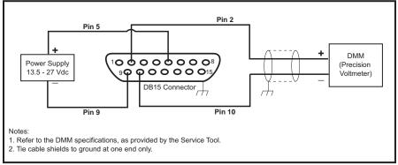
Figure 7-4 Setup for Calibrating to an Output Voltage
