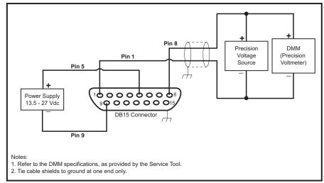
Figure 7-6 Setup for Calibrating to a Voltage Setpoint
