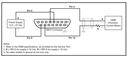
Figure 6-2 Setup for Testing Output Current
