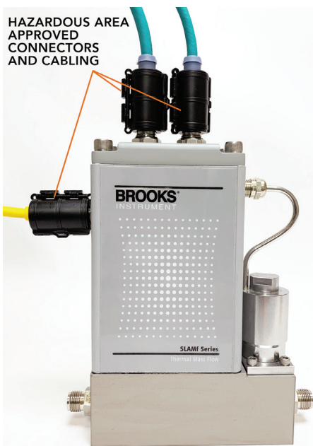
▲ Hazardous-area MFCs should have special connectors for communications and power cabling to prevent accidental disconnection when volatile substances are present.
