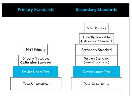
Brooks utilizes **primary standards** and the accuracy specification includes uncertainties from all reference equipment. Utilizing **secondary** and **third-level standards** increases the potential for metrology alignment issues and overall system uncertainty.
