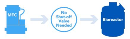
The result? One less system component needed, reduced design, testing and validation time and reduced system footprint.
